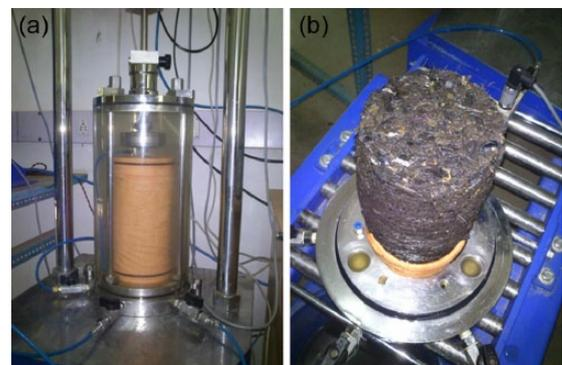
Figure 5. (a) Dynamic testing of municipal solid waste (MSW) sample in cyclic triaxial apparatus and (b) MSW sample in triaxial mould.
