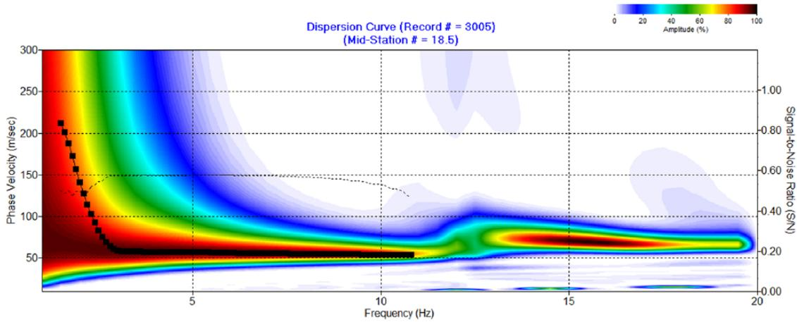
Figure 3. Typical dispersion curve from multichannel analysis of surface waves (MASW) survey.
