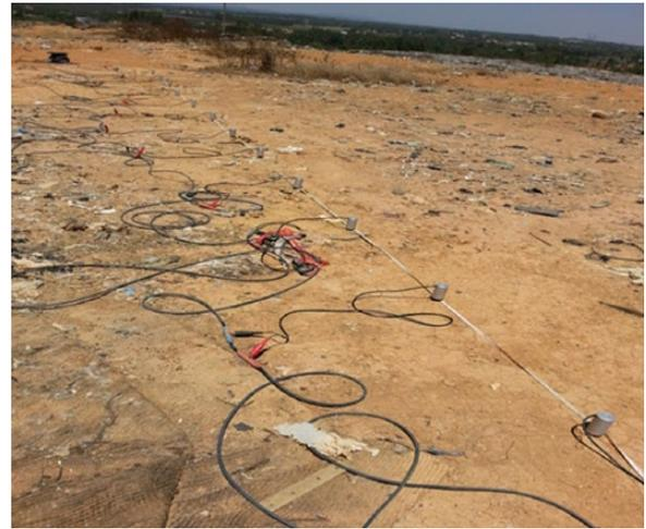
**Figure 2.** Multichannel analysis of surface waves (MASW) system geophones set-up in the municipal solid waste (MSW) fill.
