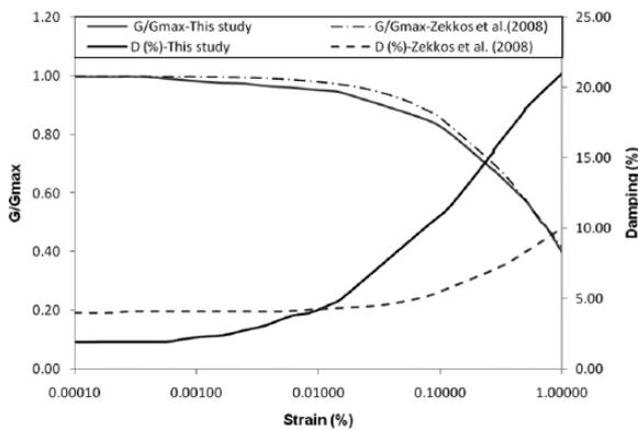
Figure 8.  $G/G_{max}$  and damping ratio curves from the present study and Zekkos et al. (2008).
