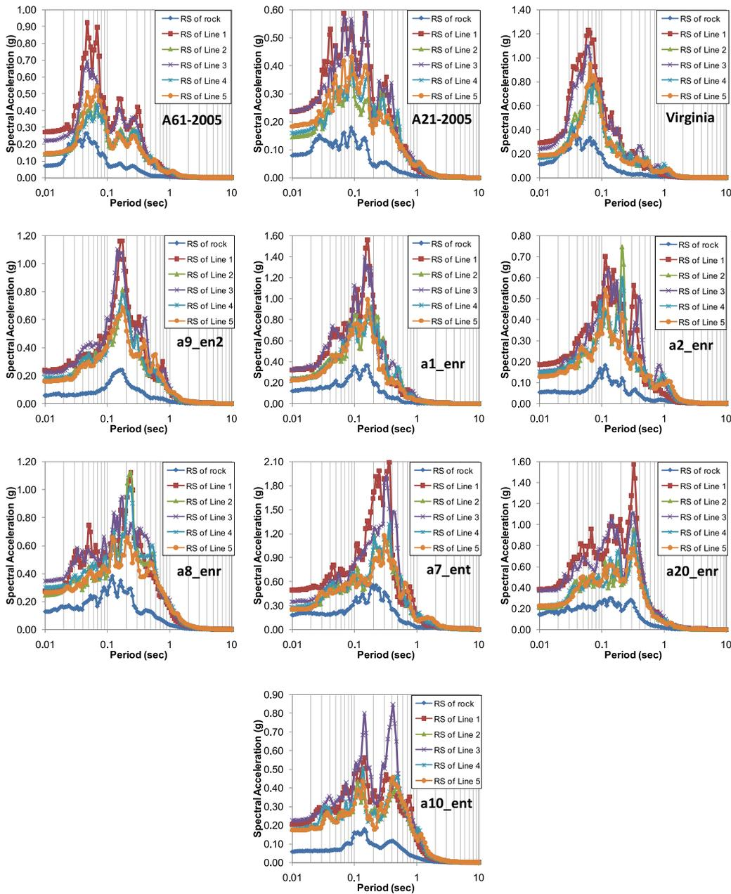
Figure 10. Input and surface response spectrum for 10 intraplate municipal solid waste (MSW) sites.
