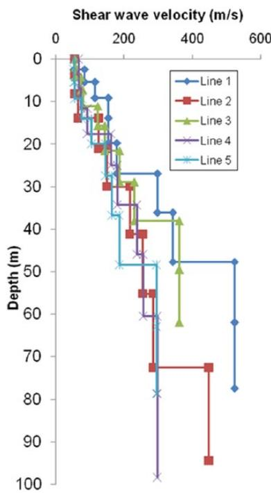
Figure 4. Shear wave velocity from multichannel analysis of surface waves (MASW) survey.
