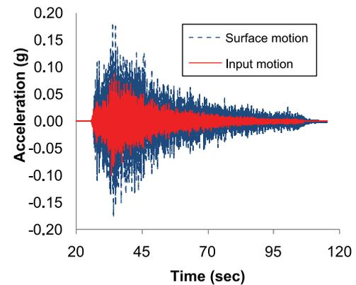
**Figure 9.** Typical input and surface ground motion for intraplate municipal solid waste (MSW) site.
