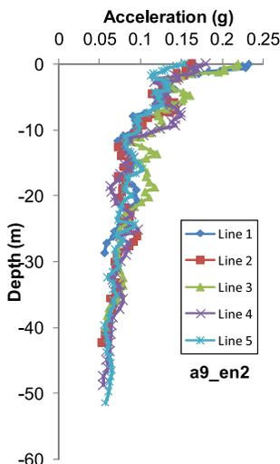
Figure 11. Typical depth versus acceleration for selected motion.
